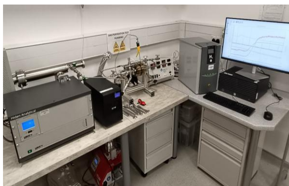
Figure 3 (left). Hiden Analytical hydrogen gas permeation set up.
