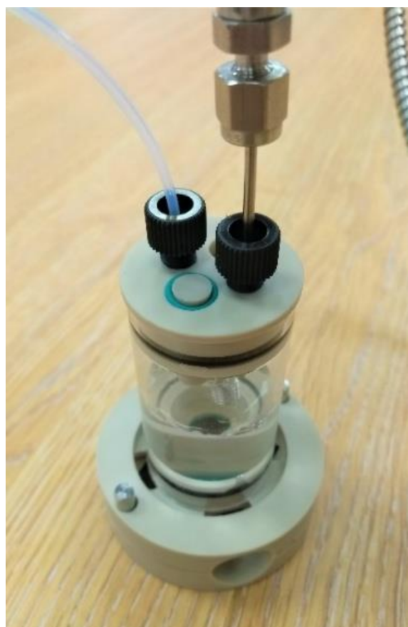
Figure 7: Ultra Low Flow capillary connected to Redox.me cell
