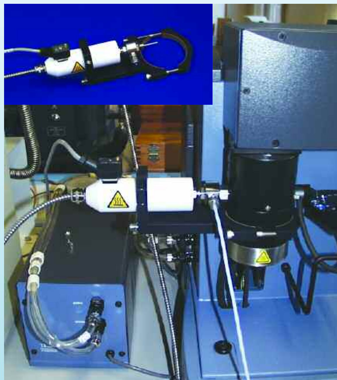
Fig 4b. TGA Interface for TA Instruments Q600 Custom designed Hot zone inlet for the TA Instruments Q500 TGA system. Includes optimised 'Hot-zone' sampling connection and heated filter assembly and support.
